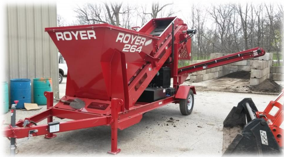
A Topsoil Processing Machine for the parks Division
