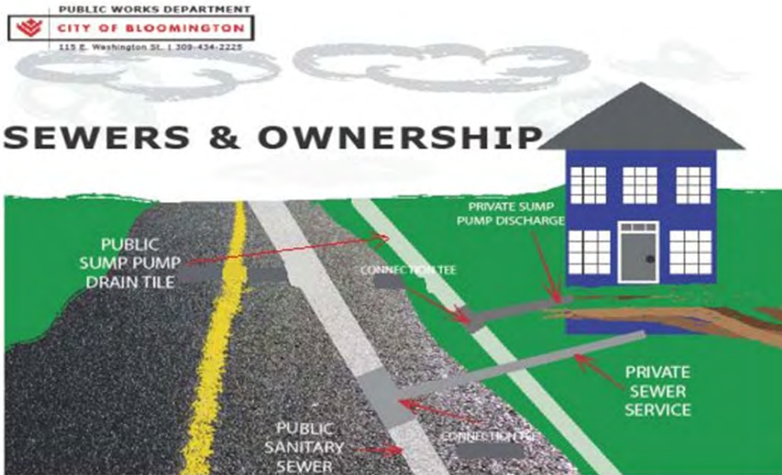
Figure 1 – Sewer and Sewer Service Ownership
