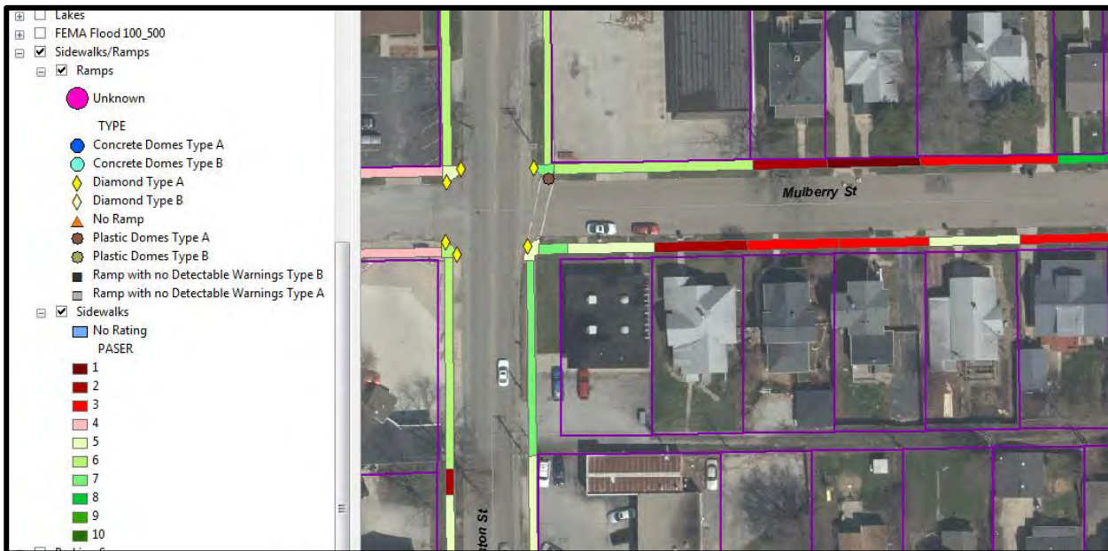
A screen shots from the Bloomington IL ArcReader application show the GIS sidewalk layer, with data for sidewalk ratings by parcel and the type of curb ramp at every crosswalks.
