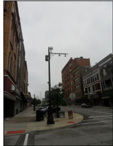
Figure 7: Camera & Wireless Access Point Pole Example
