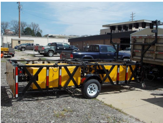
Truck Mounted Attenuator mounted on a Dump Truck
