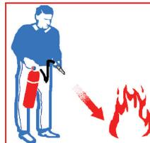
**AIM** the nozzle or hose at the base of the fire from the recommended safe distance (6 to 8 feet).
