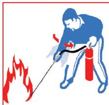
**SWEEP** the nozzle or hose from side to side until the fire is out. Continue to discharge the agent until the extinguisher is empty. Watch the area in case of re-ignition.
