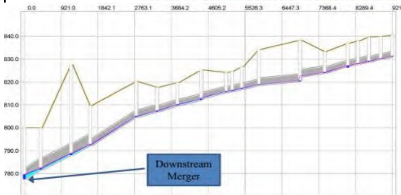
Figure 22 - Sanitary Sewer Trunk Profile
