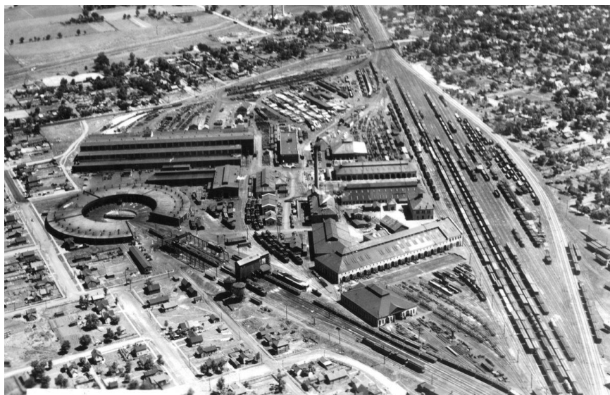
This 1931 aerial, looking north-northeast, shows the sprawling Chicago & Alton Railroad Shops on Bloomington's west side. The 44-stall roundhouse and massive locomotive backshop to its immediate northeast, were among the buildings erected in the 1911-1914 expansion project. (Photo courtesy McLean County Museum of History).
