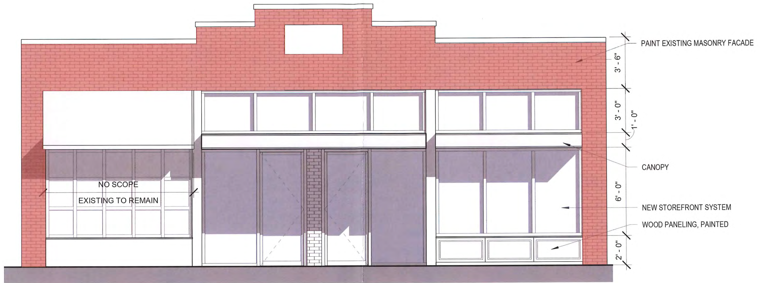
2 SOUTH ELEVATION RUST GRANT 1/4" = 1'-0"
