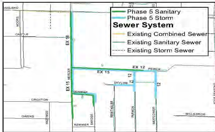
Figure 5-5 Phase 5 Proposed Sewer Improvements
