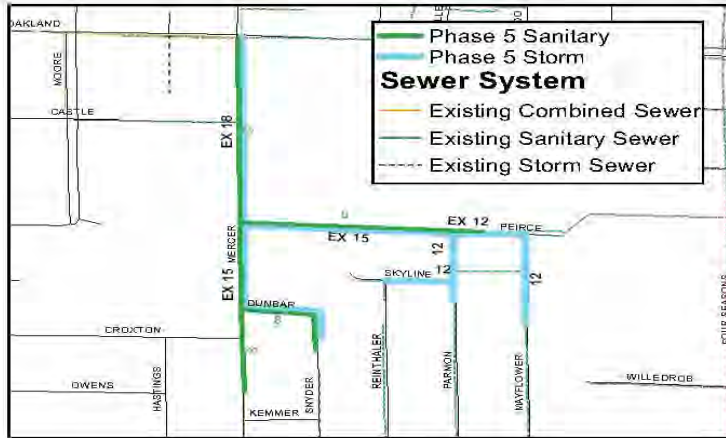
Figure 5-5 Phase 5 Proposed Sewer Improvements
