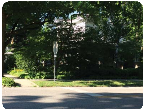
CPTED DONT's: Landscape, while defining the boundaries, is covering up natural surveillance options and providing hiding spots
