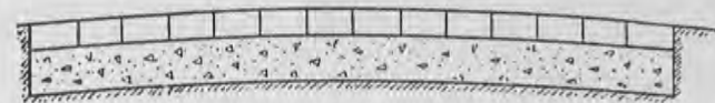
Typical monolithic brick pavement for country roads. In this type of construction, brick were laid in a wet concrete base.
