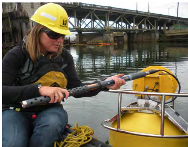
EMM68 Buoy supports a single water quality instrument, such as a YSI EXO or 6600 V2-4 Sonde, positioned inside the subsurface pipe
